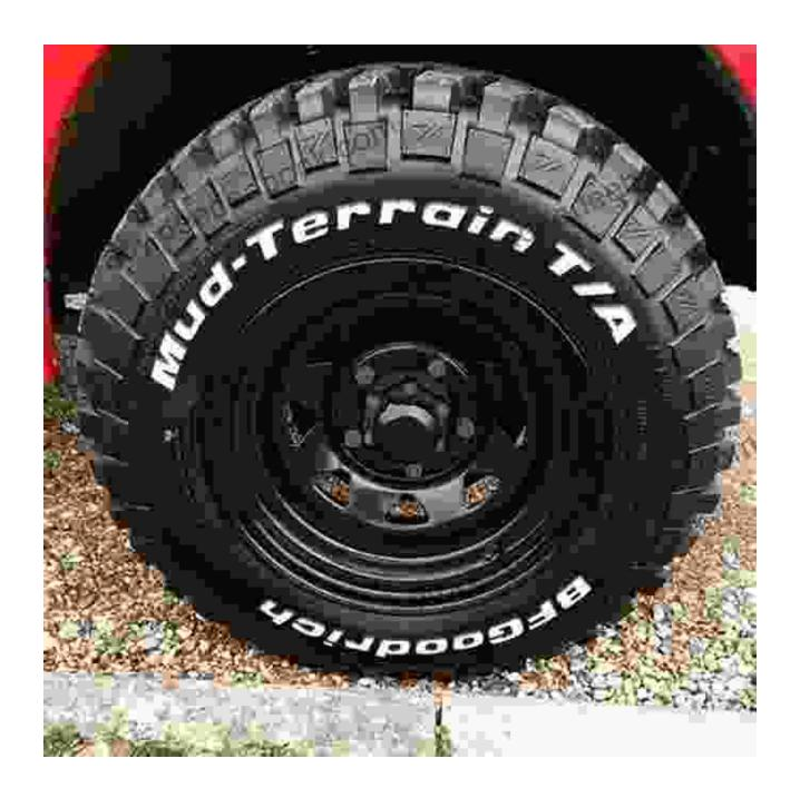
The choice of tires and wheels plays a crucial role in determining your Suzuki 4x4's off-road performance. Aggressive, off-road-specific tires with deep tread patterns provide exceptional traction on loose surfaces, mud, and rocks. Consider investing in larger tires with a higher sidewall profile to increase ground clearance and absorb bumps more effectively. Beadlock wheels ensure a secure grip on the tires, preventing them from slipping off
